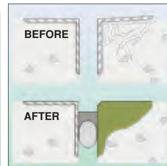
Armor Joint Repair
